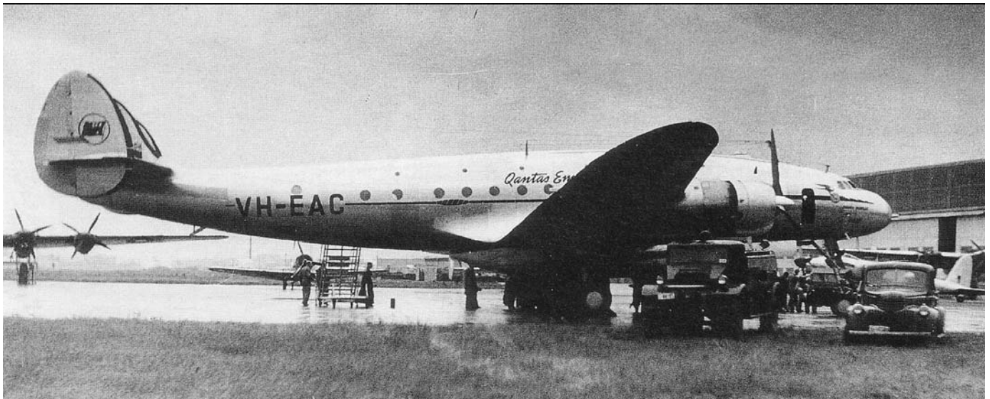
The first Constellation to carry the registration VH-EAC in 1947 being the Lockheed 749 Harry Hawker. Note the absence of wing tanks the rupturing of which exacerbated the fire following the crash. The Qantas Lockheed 1049G Super Constellation Southern Wave VH-EAC Construction No 4606 was built in 1955 (Photo: John Hopton).
