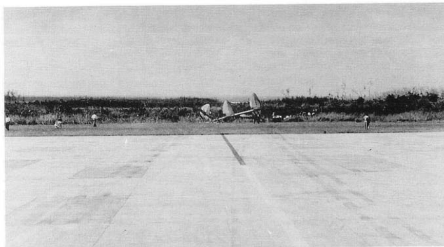
VH-EAC's skid marks can be seen leaving the concrete runway and the Constellation's triple tail fins project from the gully at the south-eastern end of Runway 13 (Photo: BASI).
