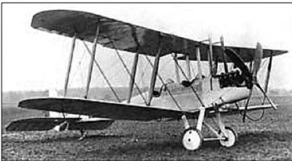
Figure 1. B.E.2 single-engine, two-seat biplane designed and developed at the Royal Aircraft Factory.
